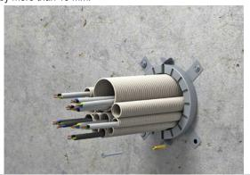
4. For reasons of smoke protection, the electrical installation conduits must be filled on both sides with GFM at a depth of at least 20 mm.
